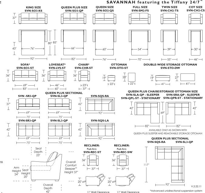
Comfort Sleepers™ utilize the Tiffany 24/7™ Convertible mechanism, U.S. Patent #4737996 and #6904628 Note: arm height for this frame is measured at the highest point of the arm
